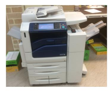
The science of static electricity is put to practical use inside a photocopier. Static electricity, however, is only one of the two scientific principles that makes a photocopier work. The other is photoconductivity.
