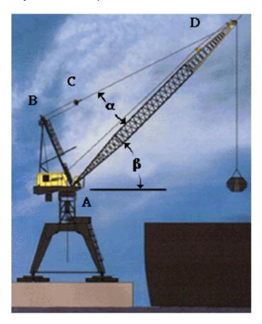
In the image, the crane is lifting an object that has a mass of 1.00 x  $10^3$  kg. The crane mast (AD) has a length of 30.0 m, with a uniform distribution of 4.00 x  $10^2$  kg mass, pivoting about point A. The mast makes an angle  $\beta$  of 40.0° from the horizontal. The cable CD makes and angle  $\alpha$  of 20.0° with the top of the crane mast (point D). Note: Angle ABD is 90.0°.
